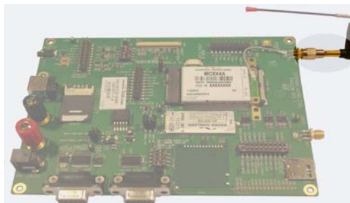
Figure 2-10: Connecting the antenna
