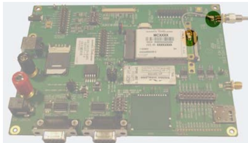
Figure 2-9: Connecting the antenna wire
