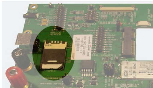
Figure 2-4: SIM inserted with cover closed
