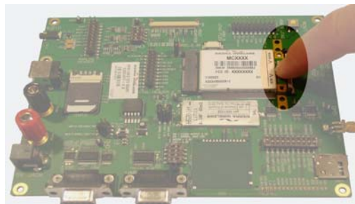
Figure 2-7: Locking a Mini Card into the Dev Kit
