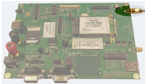
Figure 2-8: Connecting the antenna adapter
